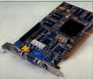
The Voodoo Banshee board is 3Dfx's second try at a single-slot 2D/3D solution, and this one just might work.
