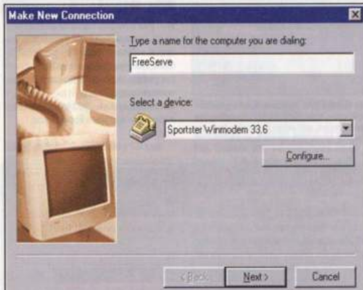
2. Type a name to describe your new connection. This is just a reminder, so you can type what you want. Make sure the device listed is your primary modem. Press Next.
