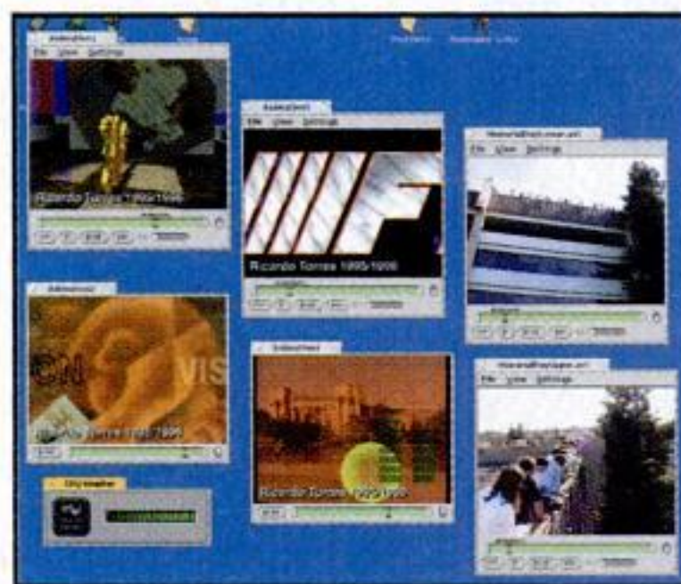
BeOS handles multiple instances of multimedia gracefully. Here, six movies are playing, all sharing sound resources, and the dual-CPU's have cycles to spare.
